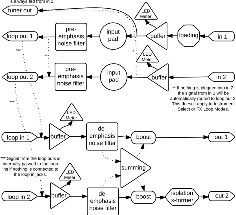
**input pads:** pads the input by either 6dB or 12dB. This can be useful for padding a very hot signal from an fx loop or active instrument. It can also be useful for matching levels from different instruments (ie. passive and active pickups, or single coil and humbucking guitars).
