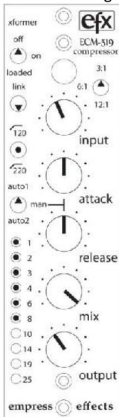
This setting is great for controlling the dynamics while tracking. The auto mode handles the attack and release times, so setup is super fast.
