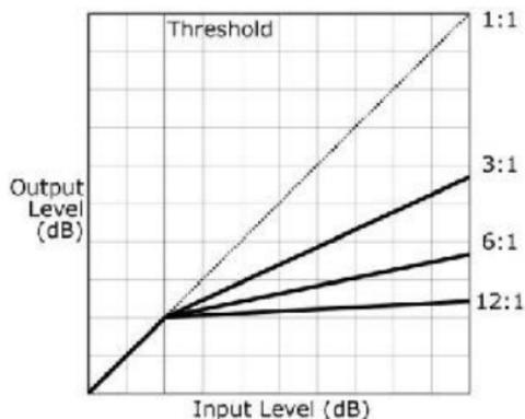
The **ratio** determines how much gain reduction will be applied to the signal once it crosses the threshold. At a 3:1 ratio, for every 3dB of input signal above the threshold, there will be 1dB of output signal. A 12:1 ratio would output 1dB for every 12dB of input signal, etc.
