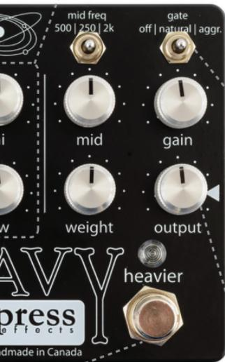
**hi:** controls the amount of high frequency content in the output signal. It is a gentle high shelf filter starting around 3 kHz. The 12 o'clock setting is 0 dB, no boost or cut, and the extreme boost and cut is about 10 dB.
