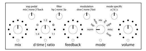
If the red bypass LED is not already lit, press the **bypass** switch to engage the Superdelay. You should hear a typical delay signal mixed with your guitar signal. You can move the knobs to suit your tastes, and change modes and sub-modes.
